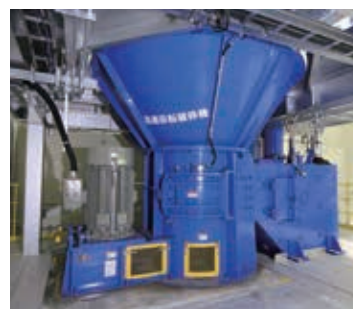
2 High-speed rotating crusher
