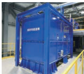
3 Magnetic separator for crushed materials
