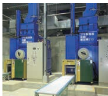
6 Plastic containers compression and packaging machine
